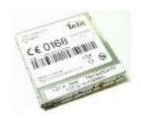
This module gets the order information from program at mini-pc and forwards orders to the dealers by SMS and/or Fax. Java runtime program generates a text file, which includes order list and location information of the user. By using GSM part of the module text file will be sent to dealer.
