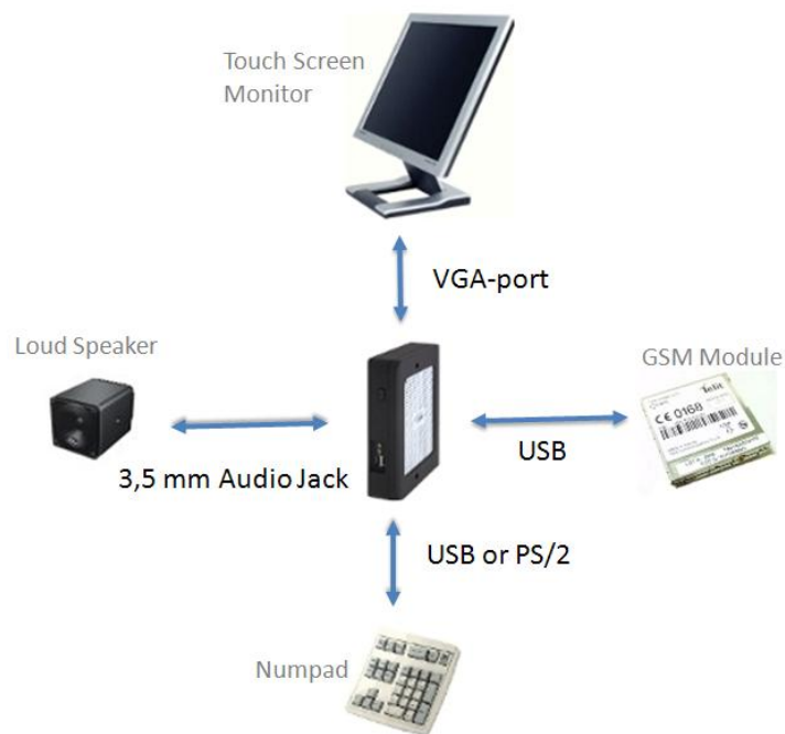
Figure 4: Product Block Diagram
