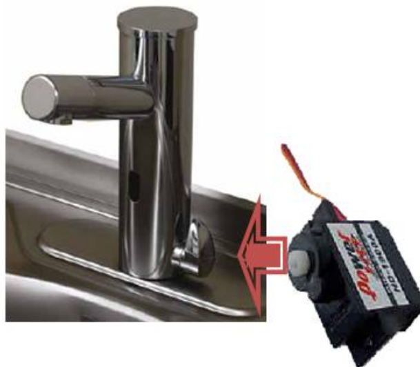
Figure 4: Electric Motor's place on faucet [3]
